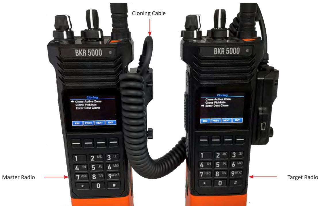
Figure 1: BKR 5000 Cloning Connections
