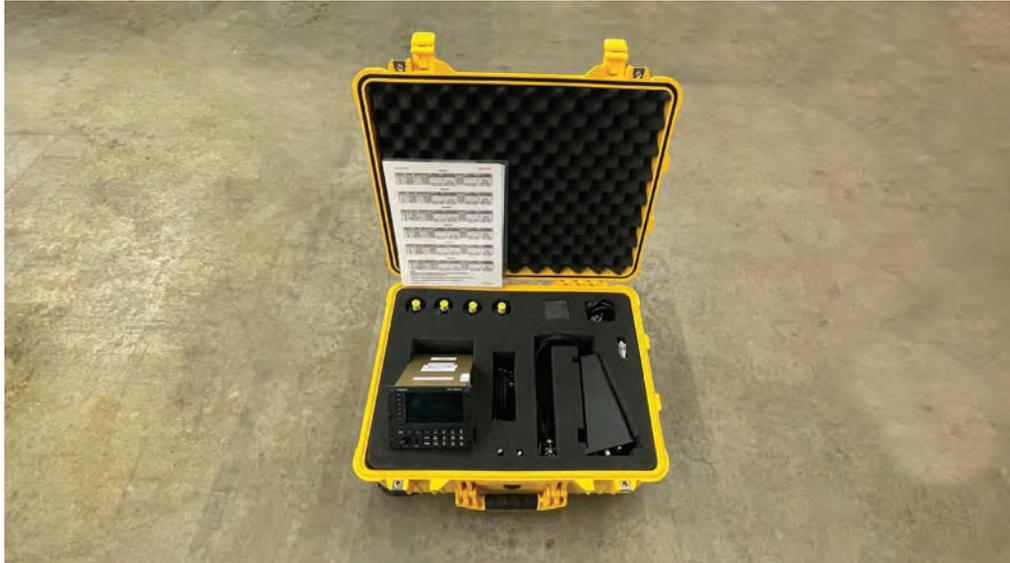
**NFES# 004605 Technisonic TDFM-136 Single Test Jig Components**
