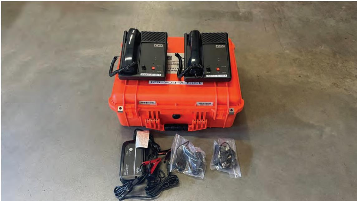
**NFES# 4330EX Remote Expansion Kit Components without NFES# 004150 Sealed Lead Acid Battery Kit**
