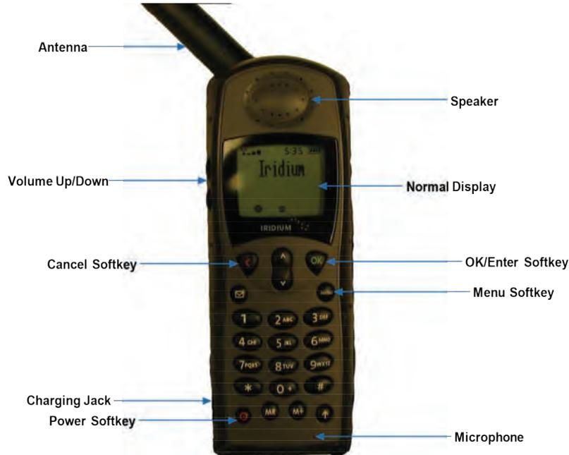
**Figure 1: 4670 Motorola Iridium Satellite Phone (Front View)**
