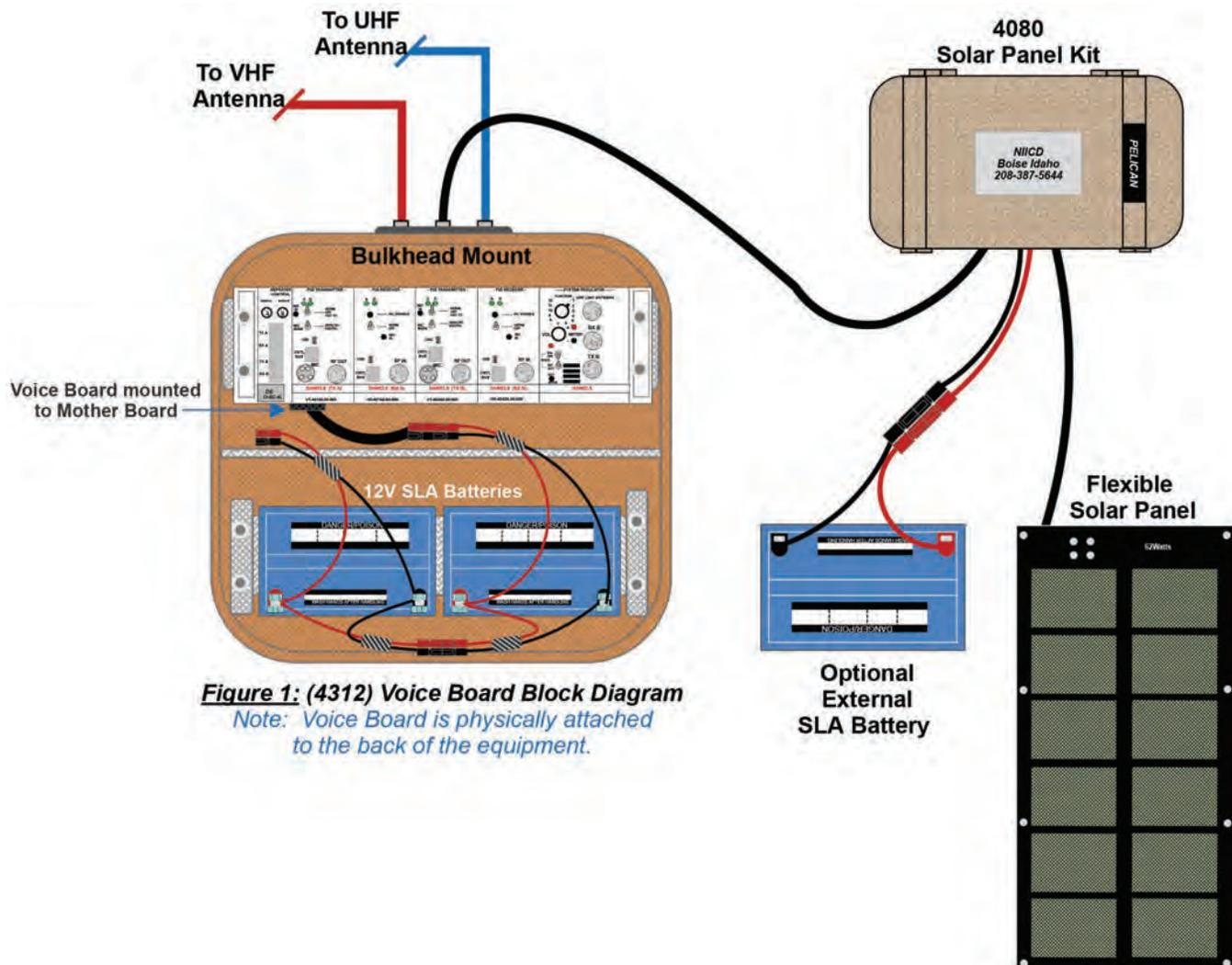
**Figure 1: (4312) Voice Board Block Diagram**
